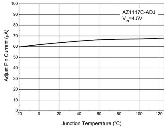
Figure 9. Adjust Pin Current vs. Junction Temperature
