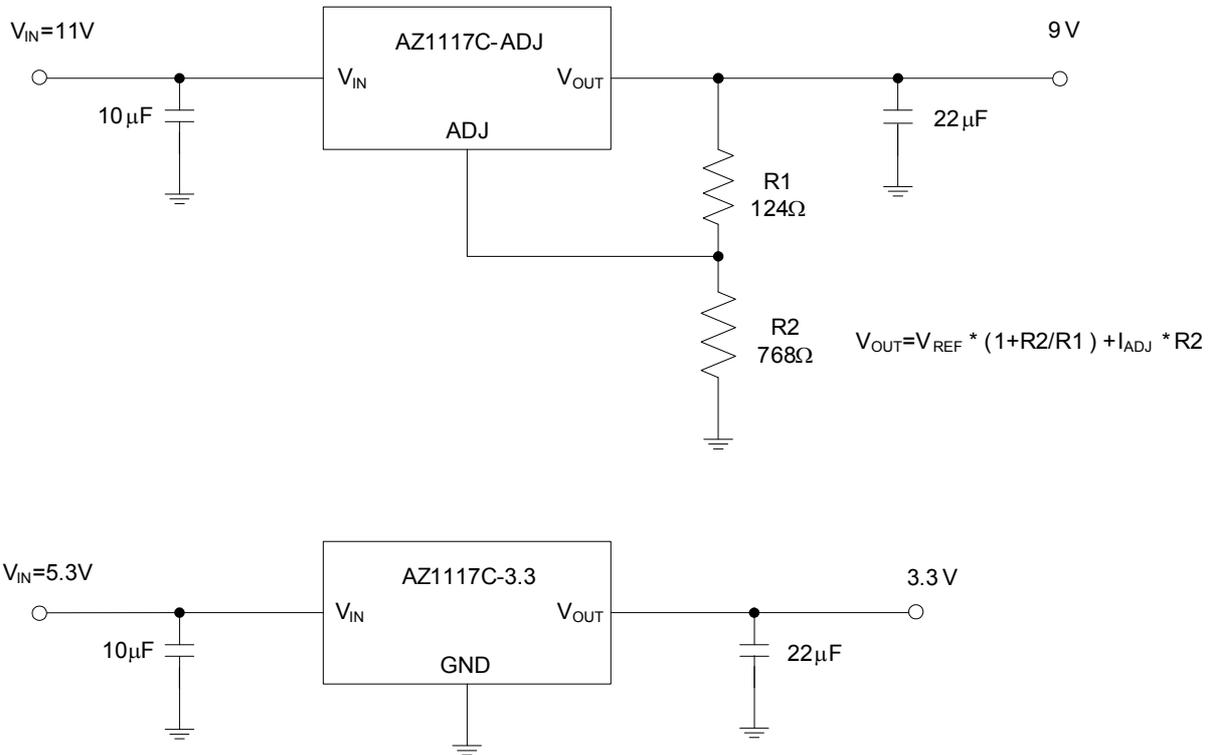
Figure 17. Typical Applications of AZ1117C
