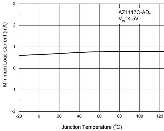
Figure 8. Minimum Load Current vs. Junction Temperature
