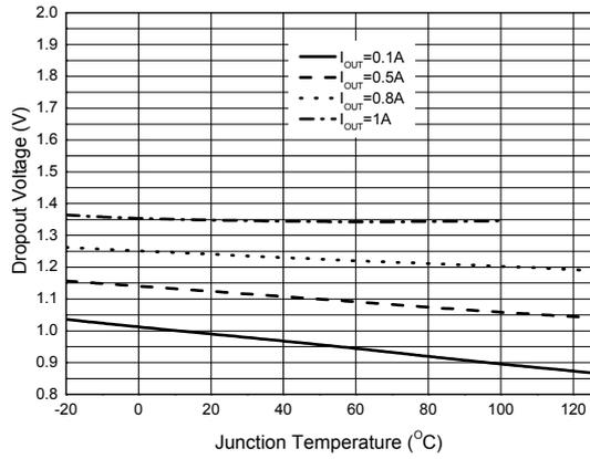
Figure 16. Dropout Voltage vs. Junction Temperature
