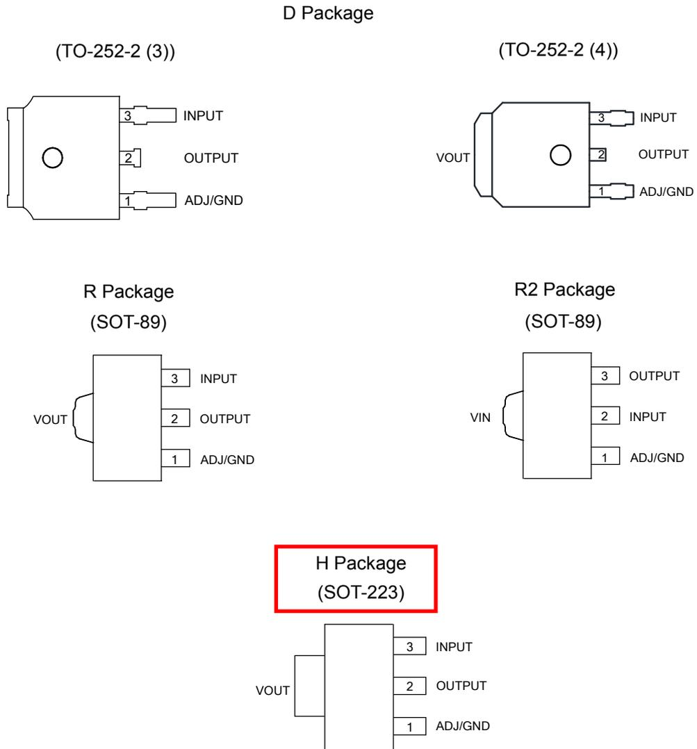
Figure 2. Pin Configuration of AZ1117C (Top View)
